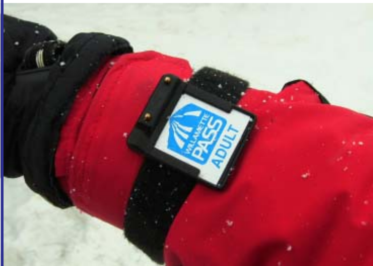
The two pins must come in contact with a sensor at the gate.
